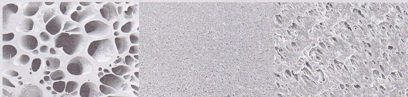
FIG. 2. Porous structure developing in PU - nanosize HA hybrids in an aqueous environment.
