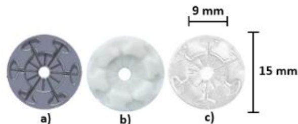
Fig. 1. a) Scaffold template design in Solidworks, b) 50% methacrylated PGSM high internal phase emulsions (HIPEs), c) 30% methacrylated transparent PGSM scaffolds.
