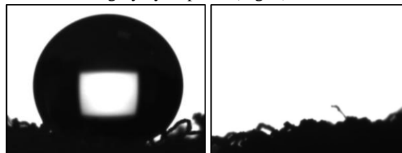
Fig. 2: Water contact angle (after 30 s) of electrospun PBS-DLS (25% w/v in chloroform, 3 mL/hr, 14 kV) Left: 96% EtOH bath. Right: 95% EtOH with 1 mM NaOH and 5 mg/mL dopamine
