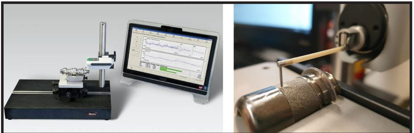
FIG. 5. The MarSurf XR measuring unit and exemplary measurement.
