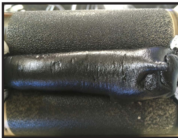
FIG. 1. Silicone matrix with carbon additive during preprocessing on a triple roller.
