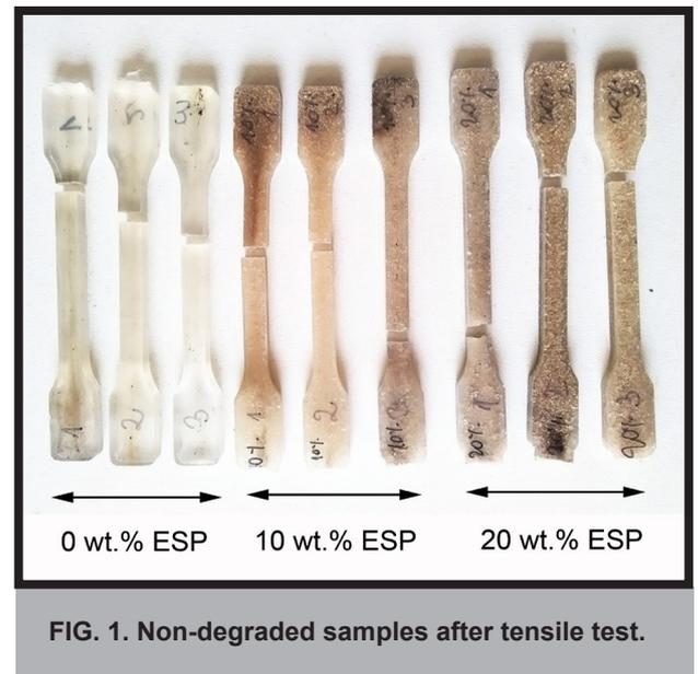
FIG. 1. Non-degraded samples after tensile test.
