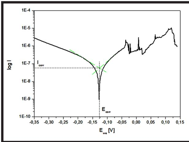
FIG. 7. The potentiodynamic polarization curve of the wire applied to the G&H Orthodontics orthodontic wire - the Ringer solution.
