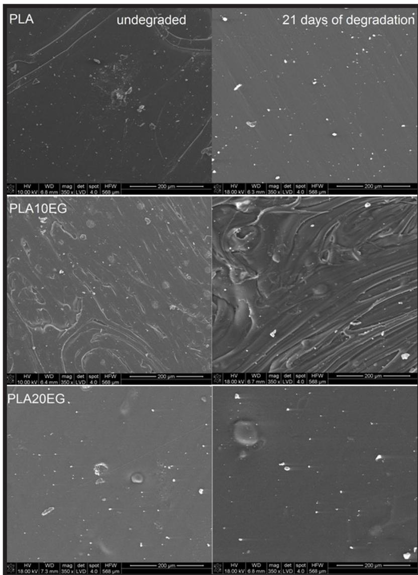
FIG. 9. SEM images of PLA-ESP samples surface before (left) and after 21-days degradation (right).
